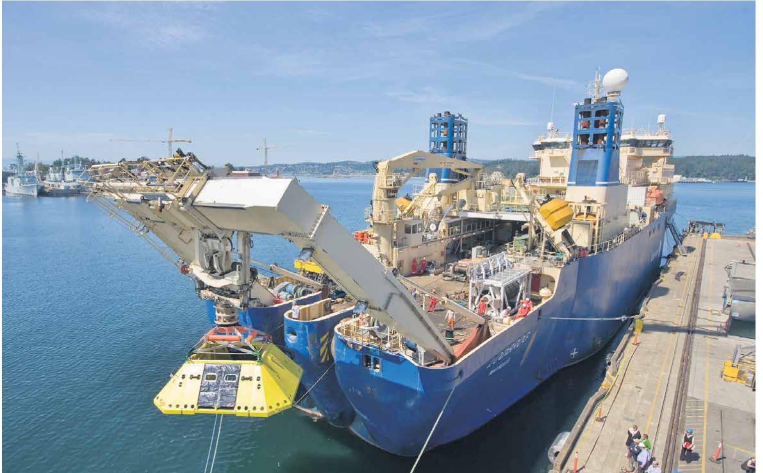
A yellow node containing a power source and Internet hub is loaded onto a ship in Victoria, B.C. The hub is part of Ocean Networks Canada, a system of hundreds of kilometres of cable attached to a raft of instruments and sensors laid along the ocean floor. The network uses the Internet to broadcast real-time data on marine life and earthquakes. OCEAN NETWORKS CANADA
