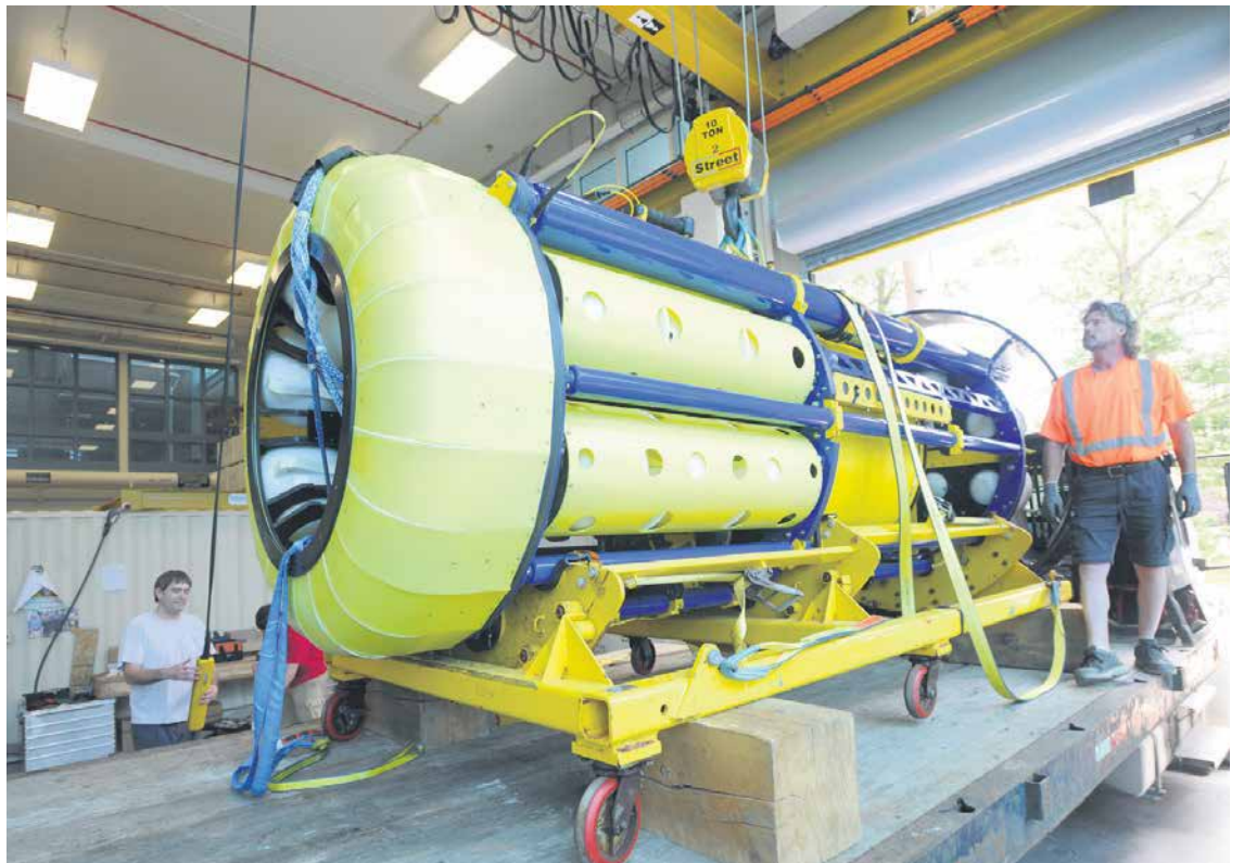
Technology like the SeaCycler, a new oceanographic mooring system with a large suite of sensors capable of collecting measurements near the surface, can help Dalhousie University researchers gain a better understanding of issues such as atmospheric gas exchange. SUPPLIED
